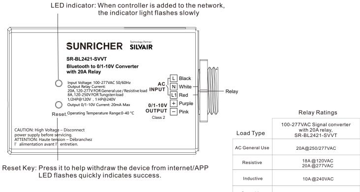
Note: 12AWG for power line; 22AWG for dimming(signal) line
